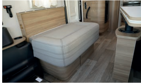
Remove the padded bench seat by freeing the rod and pulling the two guide lines upwards
