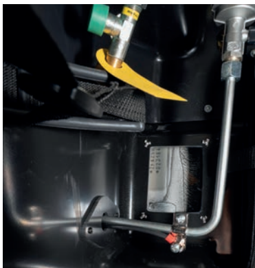
Hard stamped number is visible through front right gas bottle cupboard window.
