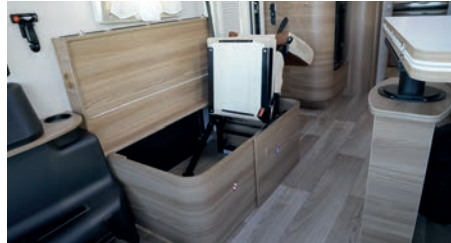
Remove the padded bench seat by freeing the rod and pulling the two guide lines upwards
