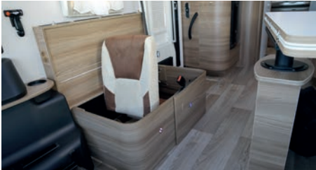
Remove the padded bench seat back
