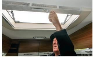
The 820mm x 520 panoramic sunroof opens with a winder and is on stays, what a great idea instead of push open and pull close - no blowing up in the wind with
