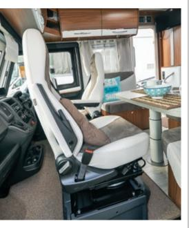
The passenger side has a large entry door; here you can see the passenger seat swivel around to complement the seating in the dining/lounge area. The table drops down to convert the dining area into a sleeping berth
