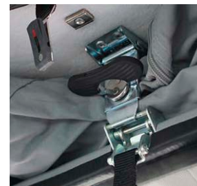
Butterfly clip that locks the roof
